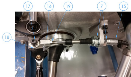
IMAGE OF SHIFT CABLE ON RIGHT SIDE OF GEARBOX
